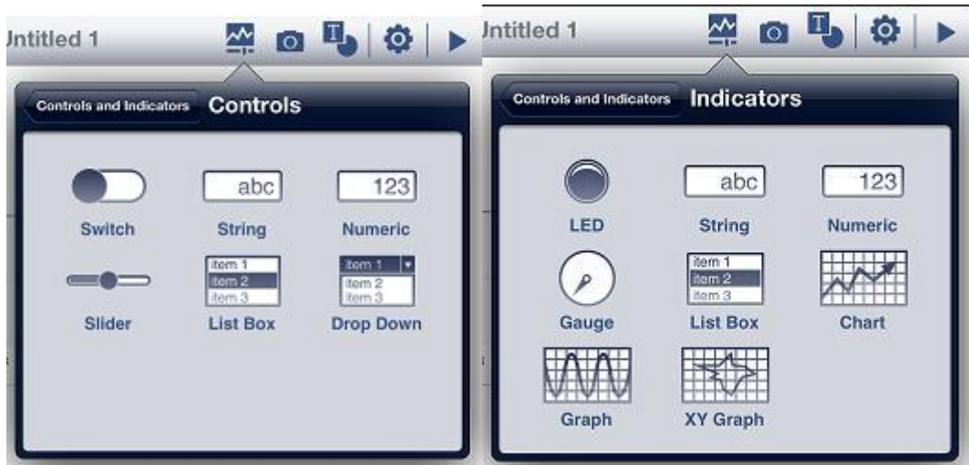
Figure 9. The controls and indicators available in Data Dashboard for LabVIEW app running on the iPad
